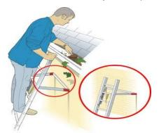
The top of the ladder rests against a solid surface; ladders should not rest on fragile or other insecure materials such as cement sheet, or plastic guttering;
